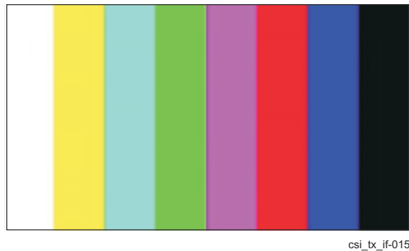
Figure 12-476. CSI_TX_IF PSI_L Color Bar sample output
