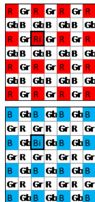
Figure 6-82. Bi-Cubic Interpolation Input Data
