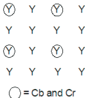
Figure 6-138. LDC Sample Grids for NV12
