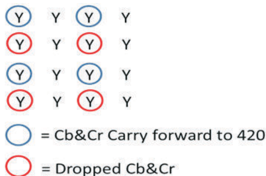
Figure 6-140. LDC YUV422 to YUV420 Conversion
